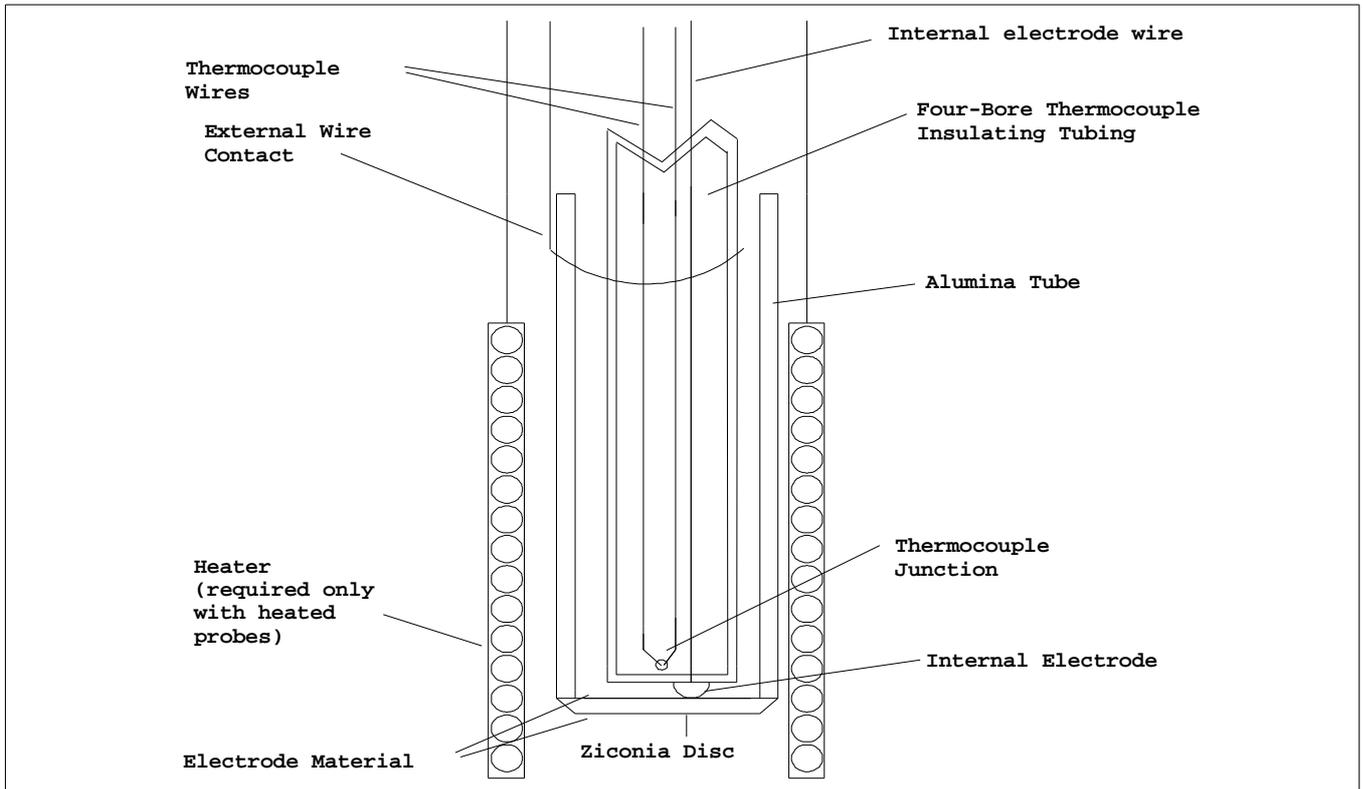
Schematic View of a Sensor Assembly
