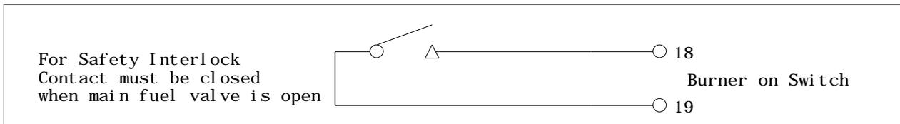
**Heater Supply Interlock Connection**
